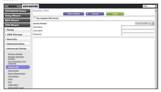
Figure 12. Forward traffic to a changing IP address
